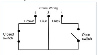
Switches shown in closed valve position. Max. cont. load 2.5 W. Insulation tested to  $1000\,\mathrm{V}$ .
